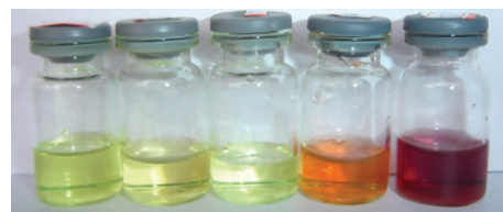
Fig. 1 Color changes observed for TBIB in water upon addition of cations. From left to right: 1: none; 2: Co 2+ ; 3: Ni 2+ ; 4: Ag + ; 5: Fe 2+ or Fe 3+ . Upon the respective addition of Na + , Ca 2+ , Mg 2+ , K + , Cd 2+ , Cr 3+ , Cu 2+ , Pb 2+ , Zn 2+ , the color is similar to 3.
